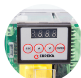
INVERTER control panel LCD programming
