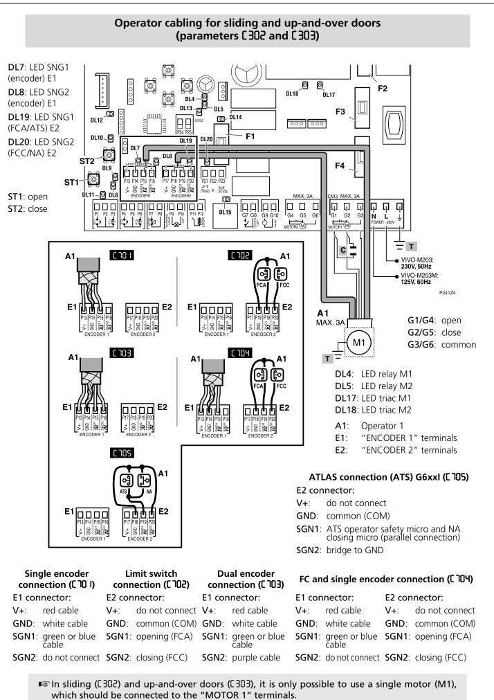
When using a single encoder (E 10 I, E 104) or dual encoder (E 103), always connect to the "ENCODER 1" terminals.
