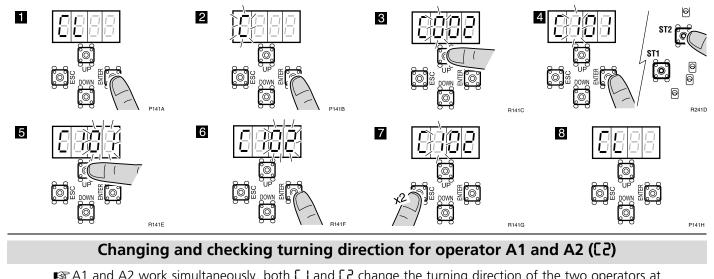
■ A1 and A2 work simultaneously, both [ ] and [2 change the turning direction of the two operators at the same time. The turning direction of a single operator cannot be changed.
