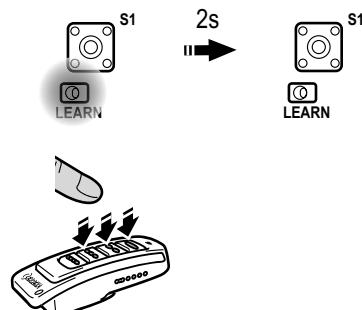
☞ Carry out the same process to programme more transmitters if required. The memory can be used with up to 25 transmitters.
