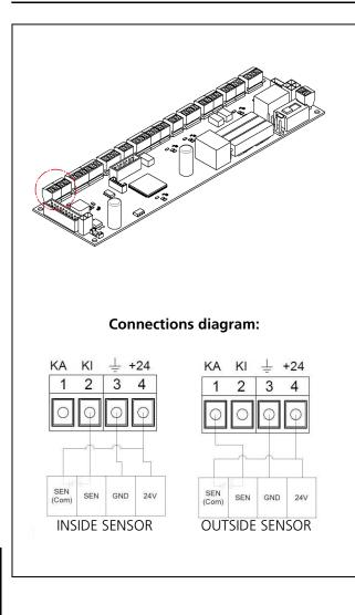
The following types of devices can be installed: radar motion sensors, passive infrared motion sensors, push buttons, switches, radio, IR receivers, access control systems, telephone and intercom systems, etc.
