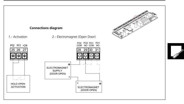
A programmable input can be configured to keep the door open using the hold-open devices.
