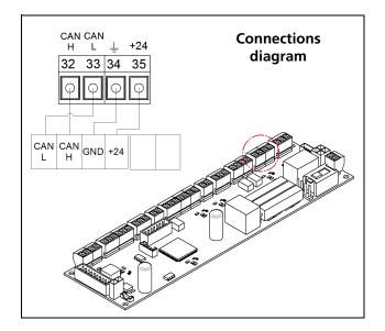
Install the Digital selector or Rotary selector according to the following connections diagram.
