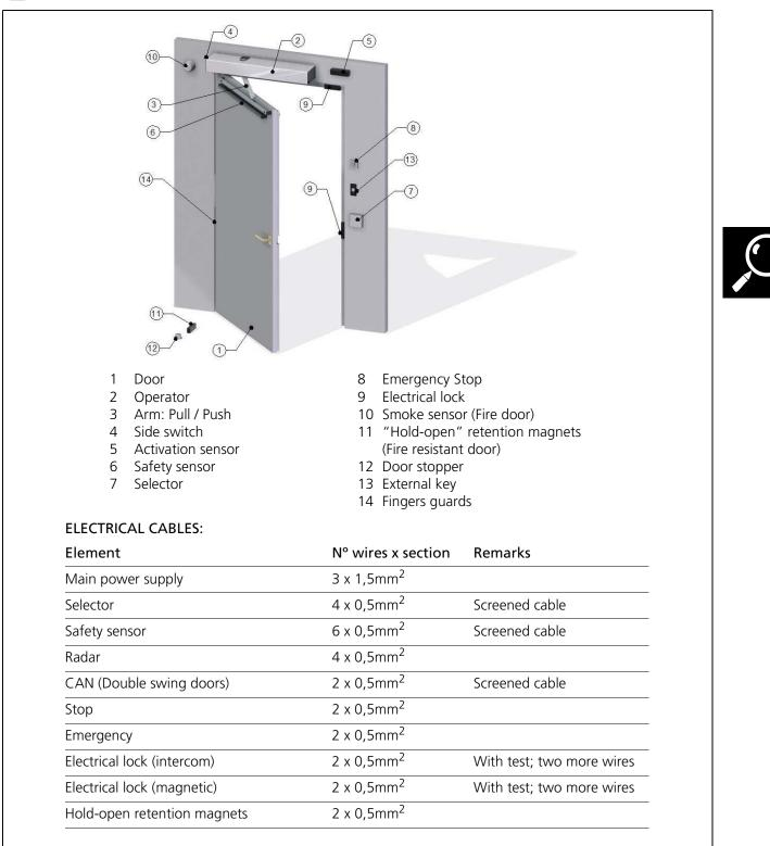
Fig. 1 Elements of the complete installation
