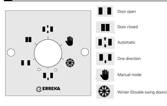
▲ To RESET, press the concealed pushbutton to the right of the exit only icon using a tipped instrument.
