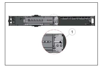
The closing force should be adjusted to each door in accordance with its characteristics. To do this, turn the screw (1) clockwise to increase closing force, or anticlockwise to reduce closing force.
