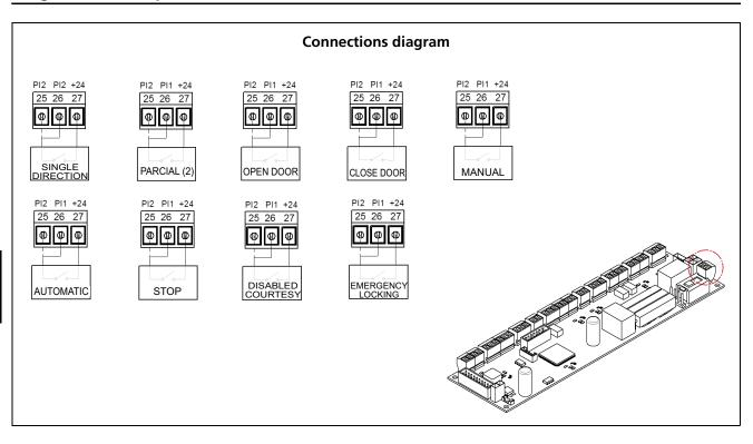
The following programmable inputs can be configured from the selector:
