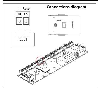
Enabling the signal directly resets the electronic plate's microprocessor.
