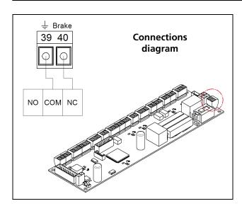
The contact must be closed to enable the passive brake. Connect as follows to install the microswitch to disable the passive brake at the end of closing.
