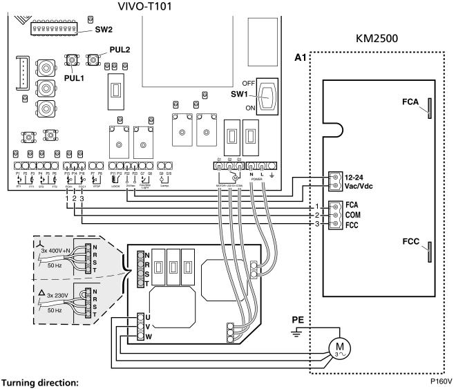
Press PUL1 and PUL2 to check the turning direction of the operator. If it is not correct, interchange the operator cables connected in cable connectors V and W.
