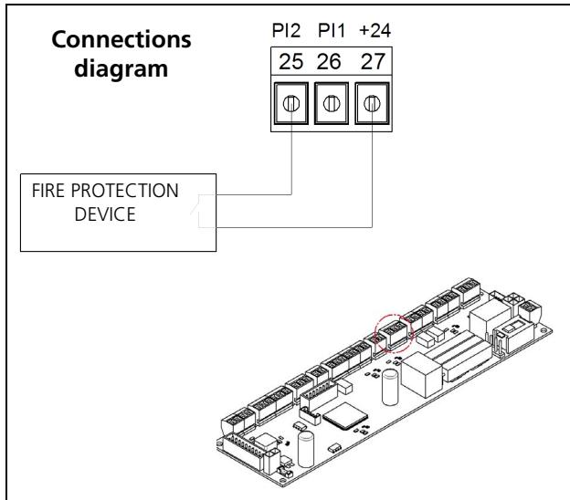
The smoke detection device (or activation signal) must be installed in doors configured as Fire Doors. Reset to restart the door.
