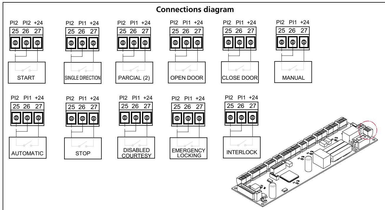
The following programmable inputs can be configured from the selector:
