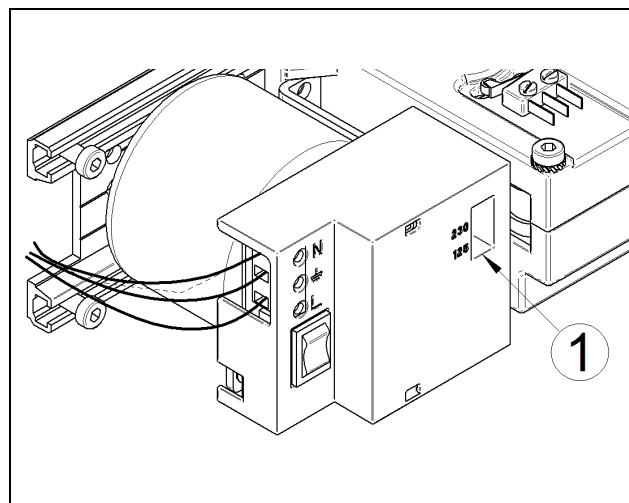
**1** Connect the line cable (L) to the bottom cable connector and the neutral cable (N) to the top cable connector.
