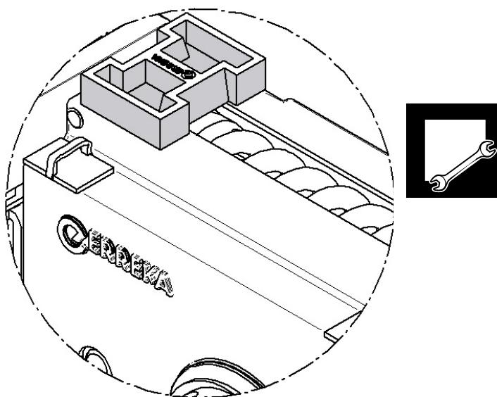
3 Release the arm. Fasten the arm again in the position it will be in with the door closed.
