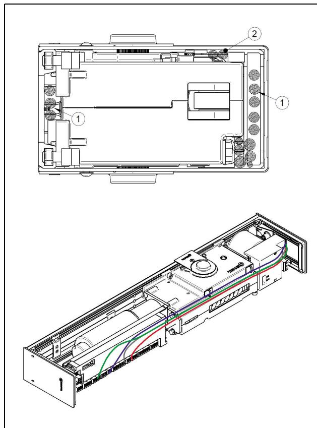
Due to the compact design of the operator, the internal wiring of the operator must be done in an orderly manner to avoid problems putting the cover on.
