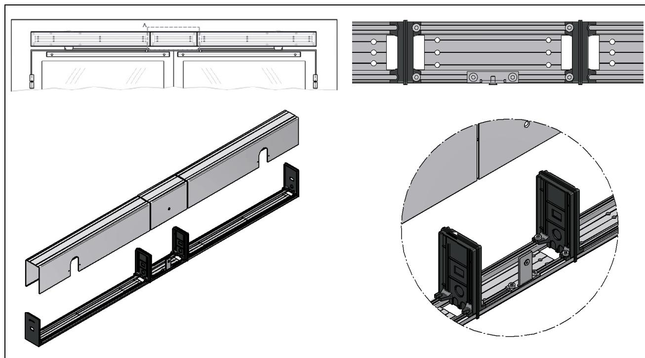
**⚠ The side covers of the operators and the intermediate casing must remain attached.**
