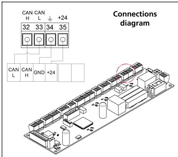
Install the Digital selector or Rotary selector according to the following connections diagram.
