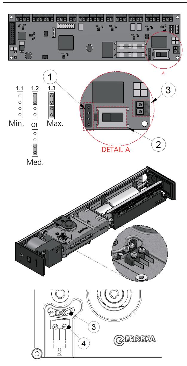
When the operator works as a door closer (manually), the motor must brakes in closing direction in order to prevent the door from gathering speed due to the force of the spring. The following must be regulated:
