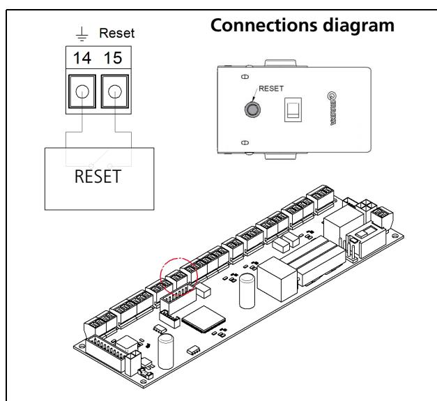
Enabling the signal directly resets the electronic plate's microprocessor. The operator will carry out the reinitialisation process, but without performing the full opening and closing sequence of the door leaf/leaves.
