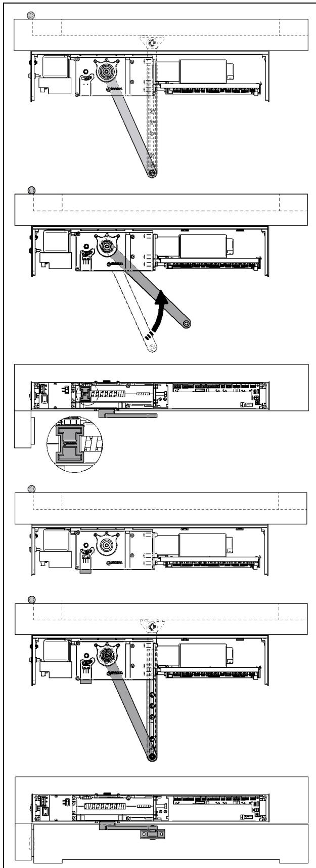
1 Fasten the arm in the position it will be in with the door closed.
