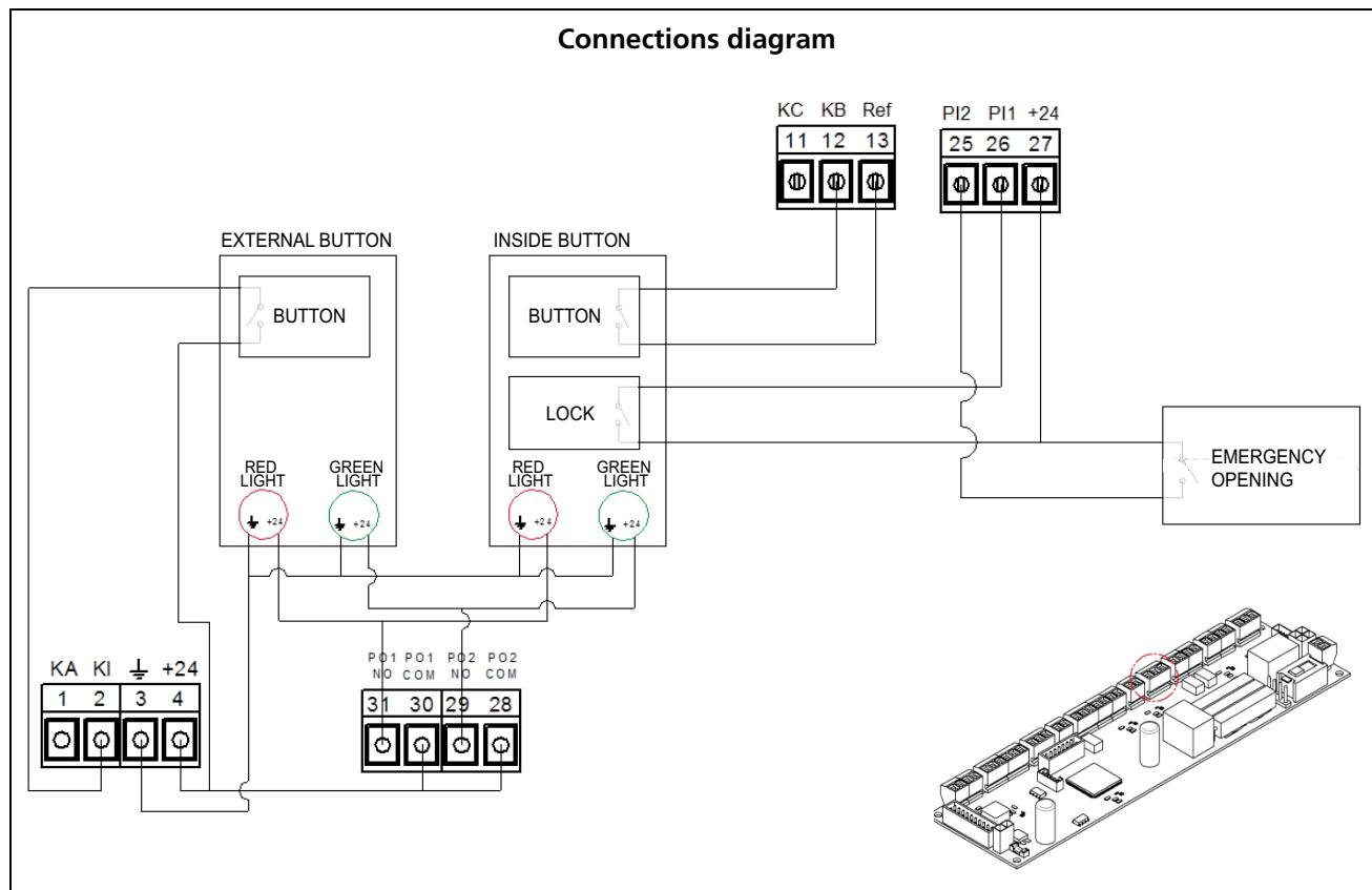
**⚠ When selecting the accessible toilets option on the selector, all necessary programmable inputs and outputs (PI1, PI2, PO1 and PO2) will be configured automatically.**
