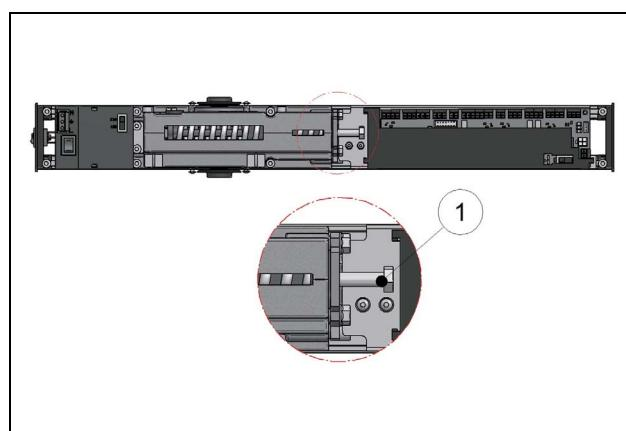
The closing force should be adjusted to each door in accordance with its characteristics. To do this, turn the screw (1) clockwise to increase closing force, or anti-clockwise to reduce closing force.
