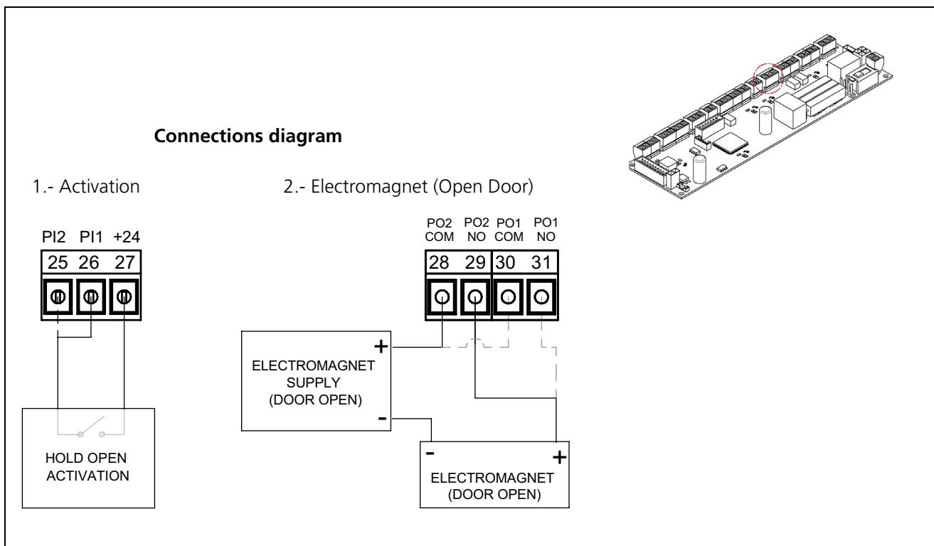
A programmable input (PI1 or PI2) can be configured to hold the door open using hold-open devices (e.g. maglocks).
