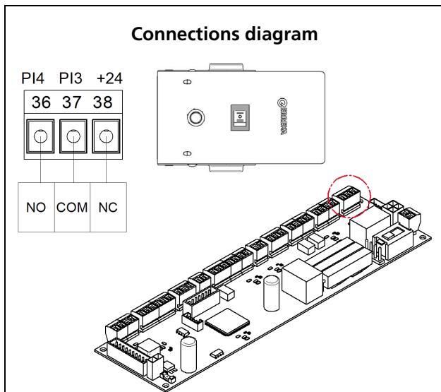
Connect the side switch cables according to the following wiring diagram.
