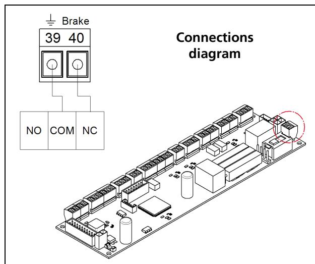
For the passive brake to operate, the contact must be closed. Connect as follows to install the microswitch to disable the passive brake at the end of closing.
