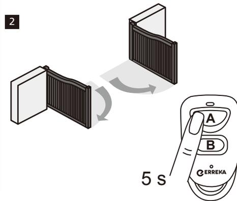
Press B button for 5 seconds for single-gate installation.
