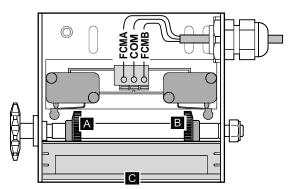
Ensure that the limit switches are connected correctly (the closing switch in the FCC cable connector and the opening switch in FCA). If this is not the case, the motor continues to work until wheel A or B reaches the stopper, causing the mechanism to break.
