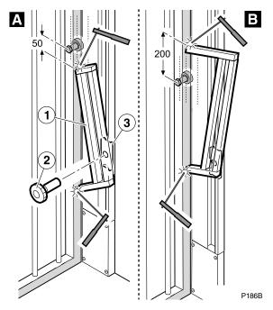
Dual drive only: install the crankshaft on the other side of the door, at the same height as the first one.
