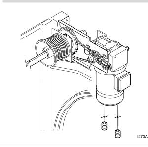
When using the SIRIUS operator (SI210DC, SI510DC, SI230DC, SI530DC only) in sectional doors, it is necessary to use adapter kit AIZ01/02 with adapter NXADAP, which is supplied separately. For further information on installing the SIRIUS operator in sectional doors, see the instructions for these adapters.
