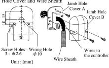
2/ Connect the wires to the door controller using the removal Terminal Block
