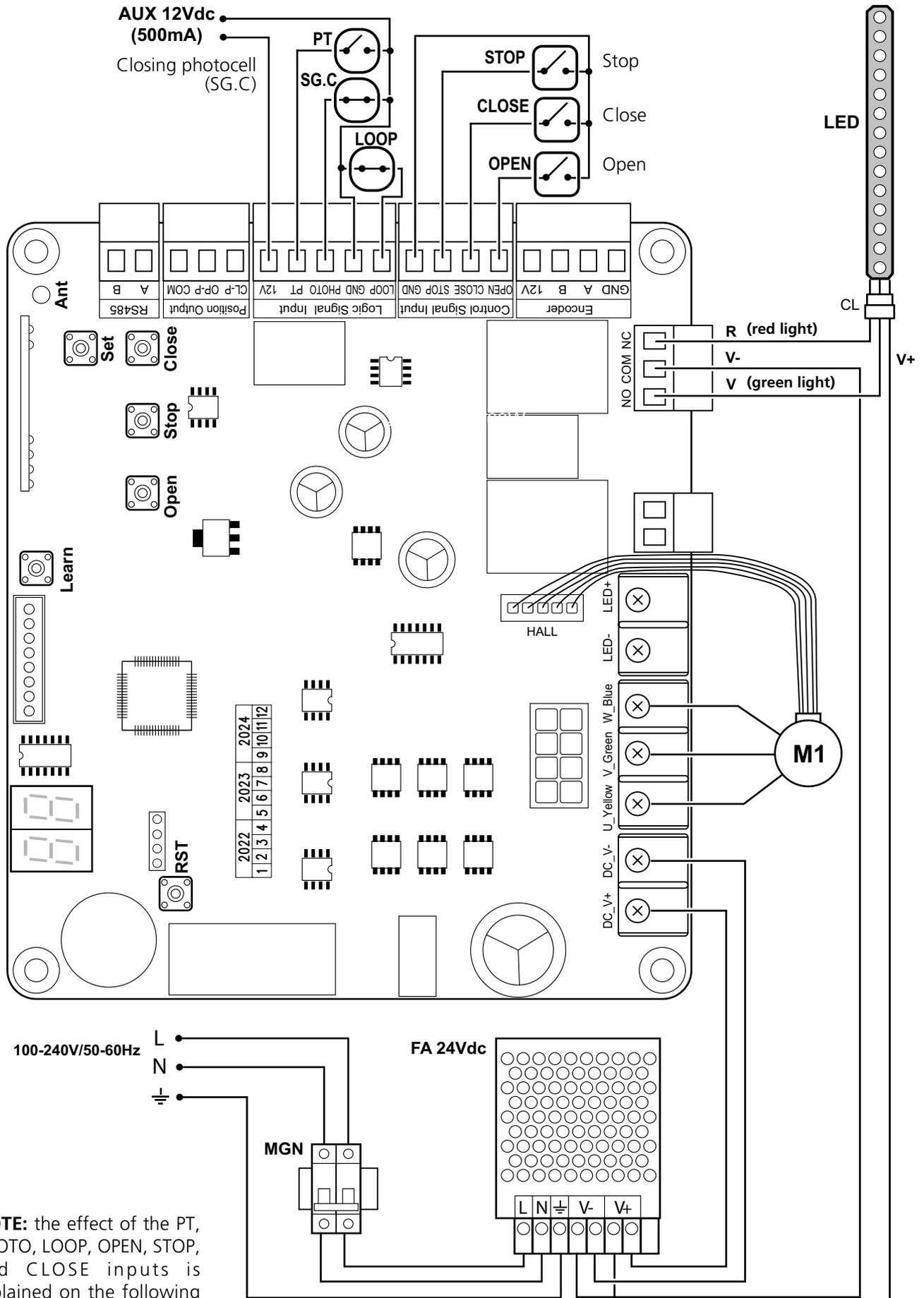
**NOTE:** the effect of the PT, PHOTO, LOOP, OPEN, STOP, and CLOSE inputs is explained on the following page.
