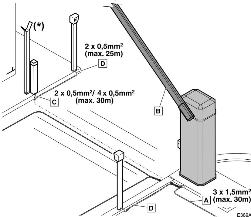
■ The diagram shows a GO PLUS right-hand barrier with LED strip.
