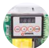
INVERTER control panel LCD programming
